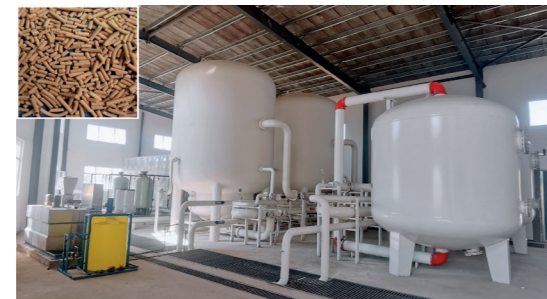
一步法除砷的非均相氧化-吸附材料与设备 Heterogeneous oxidation-adsorption materials and facilities for one-step arsenic removal
